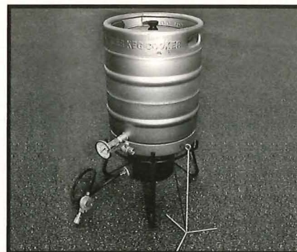
The standard "lasts-a-lifetime" setup for brewing: a converted keg heated with a Cajun cooker.
