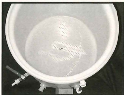
This plastic mash/lauter tun offers nearly all the advantages of stainless steel at a fraction of the cost.
